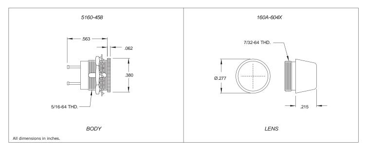
5160-458 Gem lite Indicator Light is a versatile design capable of accepting all T-1 sub-midget flange-based lamps. These high-quality indicators provide reliable service in a vast array of military and commercial applications where a miniature relampable front panel indicator is required. The lamp is not included with this indicator light.
