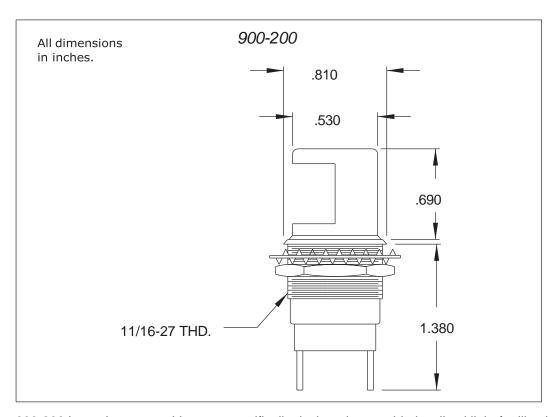
900-200 Lamp Instrument Lites are specifically designed to provide localized light for illuminating panels, meters, switches and legends. The Lamp Instrument Lite features a highly reflective surface on the inside of the hood to assure peak light output and is easily re-lamped from the front of the panel. The lamp is not included with this indicator light; order the required lamp separately.
