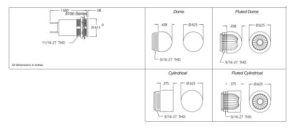
The 5100 Series Miniature Indicator Lights are versatile, industry standard, front panel indicators capable of accepting a variety of T-2 and T-3 1/4 miniature bayonet based incandescent and neon lamps. These indicator lights accept a variety of different lens styles and colors, and are excellent for providing a large, bright, easily noticed status indicator. The lamp is not included with this indicator light; order the required lamp separately.
